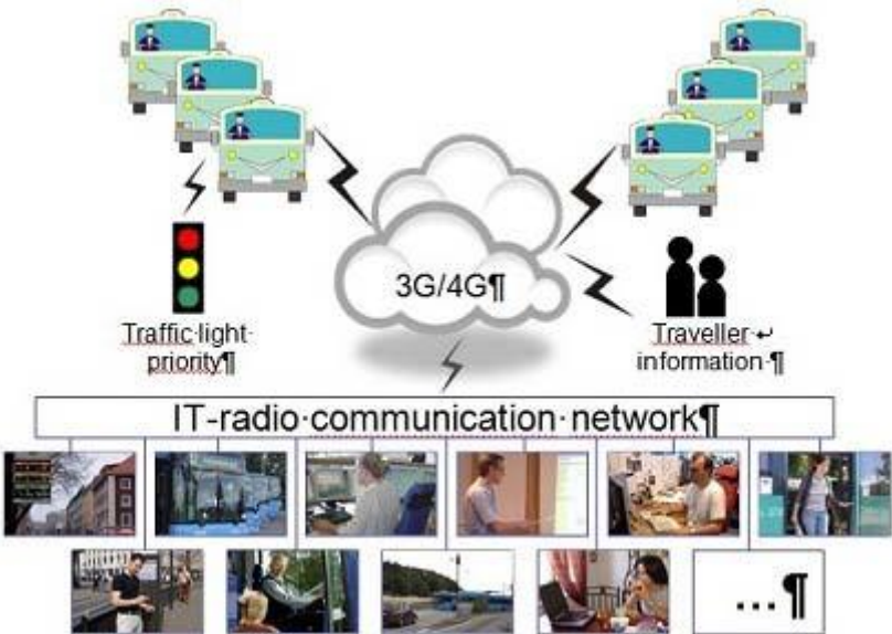
Figure 5 General communication principles between PT vehicle, central server and passenger information systems
